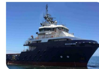
These vessels are built to provide towing services to relocate and support offshore installations. They are designed to deploy and recover mooring systems for deepwater drilling rigs and offshore floating wind installations, undertake traditional supply duties in support of drilling operations and support subsea construction activities.
