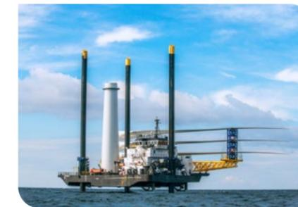
These vessels provide a self-propelled, stable platform to perform offshore wind farm installation and maintenance, production platform construction, inspection, maintenance and removal, well intervention and work-over, well production enhancement, well plug and abandonment, pipeline installation and maintenance and diving operations. SEACOR Marine operates one of the industry's largest fleets of modern liftboats.
