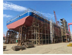
Left: Hull Erection for Hull MW628-11
