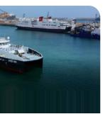
These vessels are an integral component of the logistics chain for offshore drilling rigs, platforms and other installations due to their speed, versatility and ability to carry up to 150 passengers at a time. These vessels offer a more environmentally sound, safe, cost-efficient, comfortable and flexible alternative to helicopter transportation of passengers.
